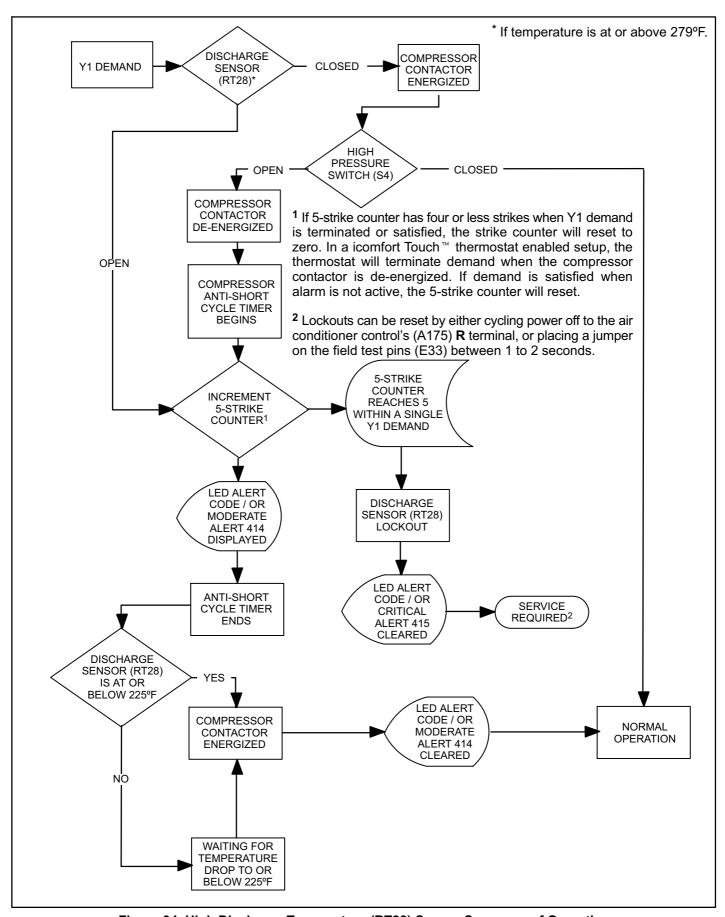
Figure 34. High Discharge Temperature (RT28) Sensor Sequence of Operation
