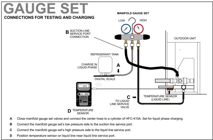
Figure 13. Gauge Set Setup and Connections
