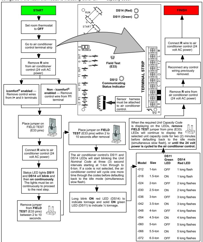
Figure 26. Main Control (A175) Unit Nominal Capacity Code Configuration (XC21-XXX-230-04 and 05)
