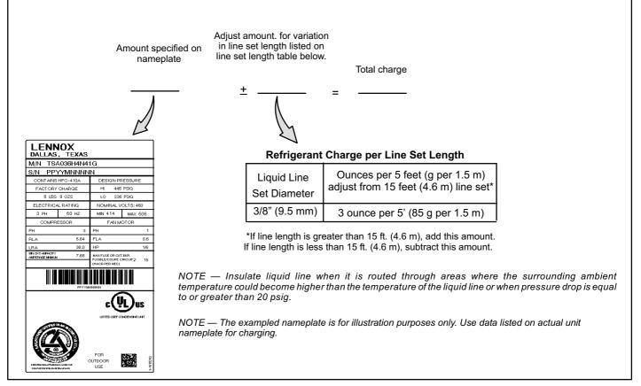
Figure 16. Using HFC-410A Weigh In Method (all builds)
