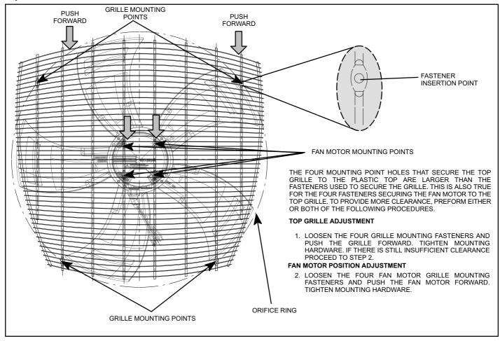
Figure 25. Fan Blade Clearance Adjustment — XC21-XXX-230-05 AND LATER
