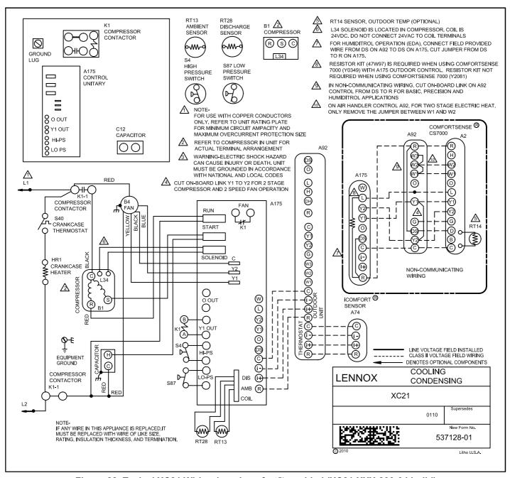
Figure 28. Typical XC21 Wiring (non-icomfort™ enabled (XC21-XXX-230-04 build)
