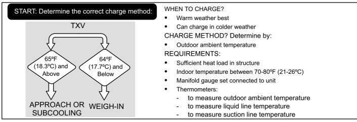
Figure 15. Determining Charge Method
