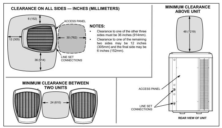
Figure 3. Installation Clearances
