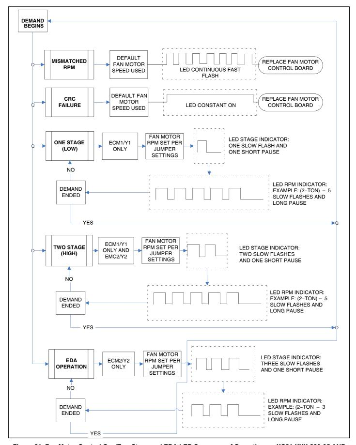
Figure 21. Fan Motor Control One/Two Stage and EDA LED Sequence of Operation — XC21-XXX-230-05 AND LATER
