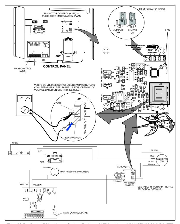
Figure 22. Fan Control, Wiring, Jumper Settings, Testing and LED Location — XC21-XXX-230-05 AND LATER
