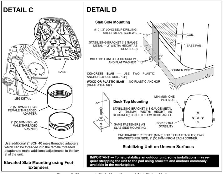
Figure 5. Placement, Slab Mounting and Stabilizing Unit
