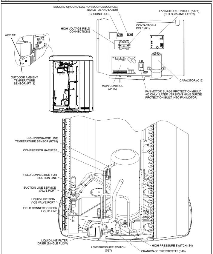
Figure 1. Plumbing, Switches and Sensor Components
