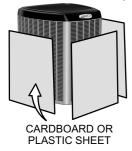
BLOCK OUTDOOR COIL: [sometimes necessary with lower temperatures] Use cardboard or plastic sheet to restrict the airflow through the outdoor coil to achieve pressures from 325-375 psig (2240-2585 kPa). Higher pressures are needed to check charge. Block equal sections of air intake panels and move coverings sideways until the liquid pressure is in the above noted ranges.
