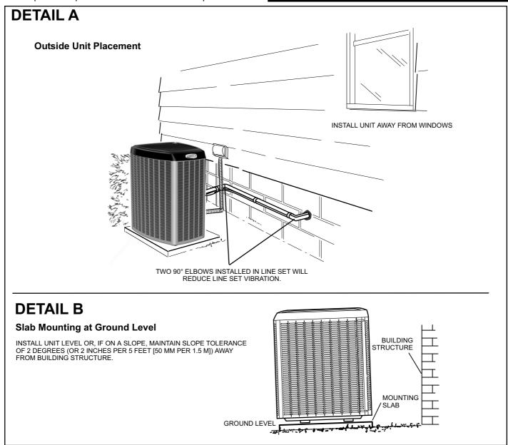
Figure 4. Placement, Slab Mounting and Stabilizing Unit
