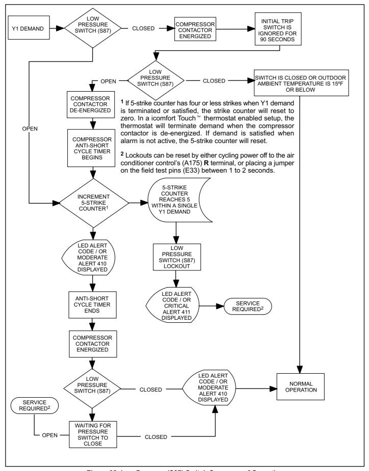
Figure 32. Low Pressure (S87) Switch Sequence of Operation
