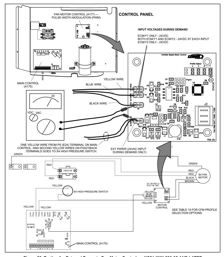
Figure 23. Testing for External Power to Fan Motor Control — XC21-XXX-230-05 AND LATER
