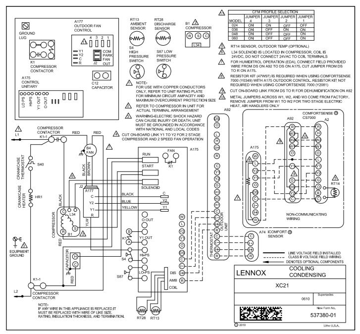
Figure 30. Typical XC21 Wiring (with icomfort™ enabled, New Fan Motor with built-in surge protection and External Surge Protection Device Removed (XC21-XXX-230-06 build)
