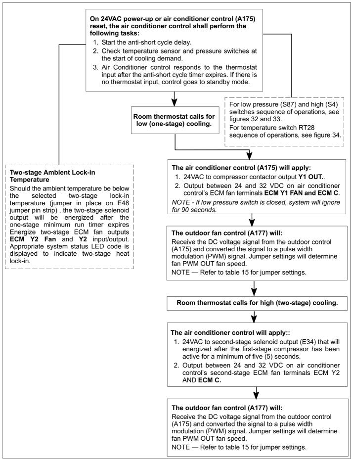
Figure 31. One-Stage and Two-Stage Cooling Sequence of Operation
