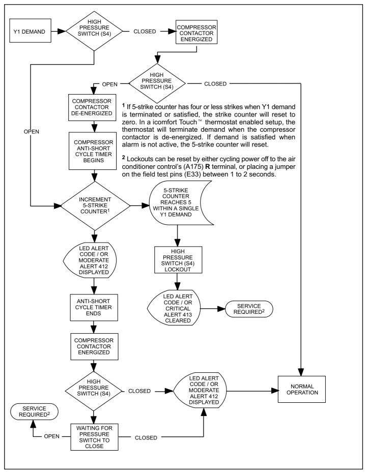
Figure 33. High Pressure (S4) Switch Sequence of Operation
