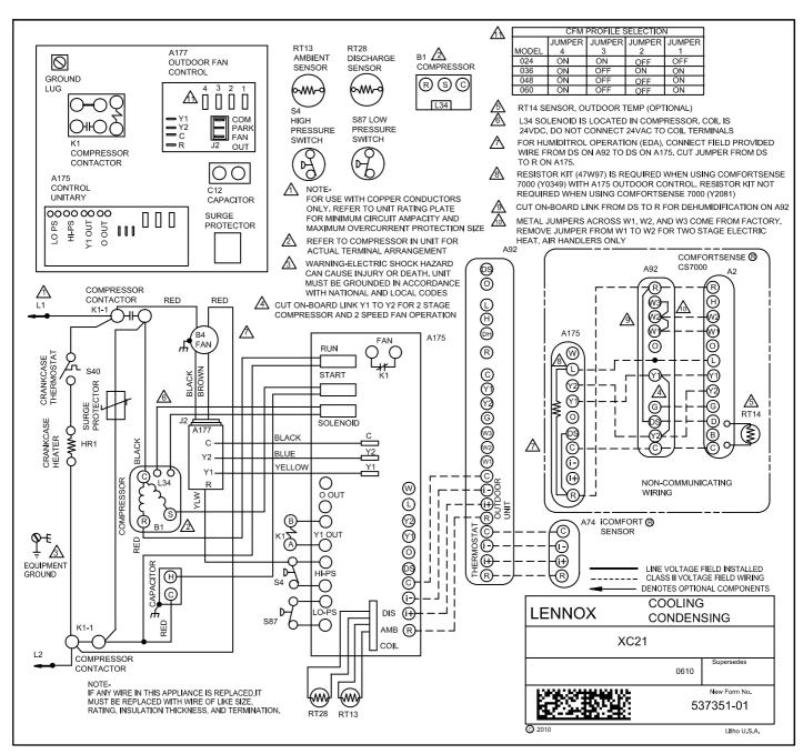
Figure 29. Typical XC21 Wiring (with icomfort™ enabled, Surge Protection and Fan Motor Control (A177) Rewired) (XC21-XXX-230-05 build)
