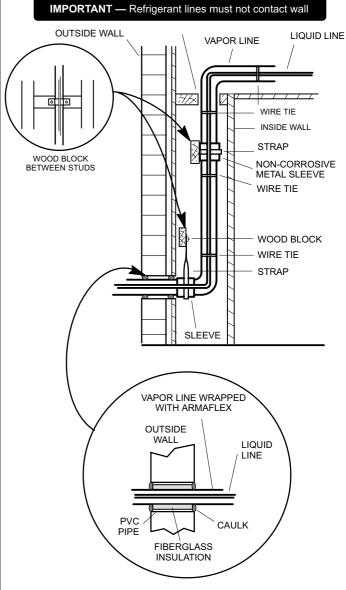
Figure 7. Line Set Installation
