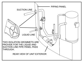
Figure 10. Isolation Grommets
