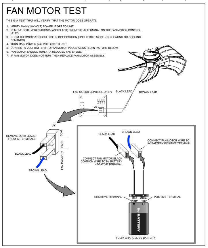
Figure 24. Fan Motor (B4) Test — XC21-XXX-230-05 AND LATER
