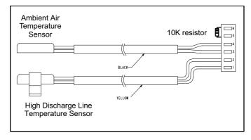
Figure 19. 10k Resistor Location
