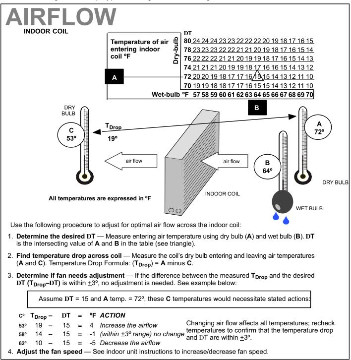
Figure 15. Checking Indoor Airflow over Evaporator Coil using Delta-T Chart
