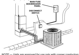
NOTE — Units are approved for use only with copper conductors. Ground unit at disconnect switch or to an earth ground.
