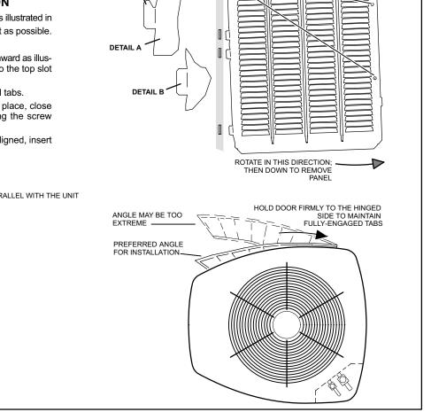
Figure 5. Removing and Installing Panels
