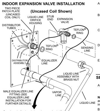
Sensing bulb insulation is required if mounted external to the coil casing. sensing bulb installation for bulb positioning.
