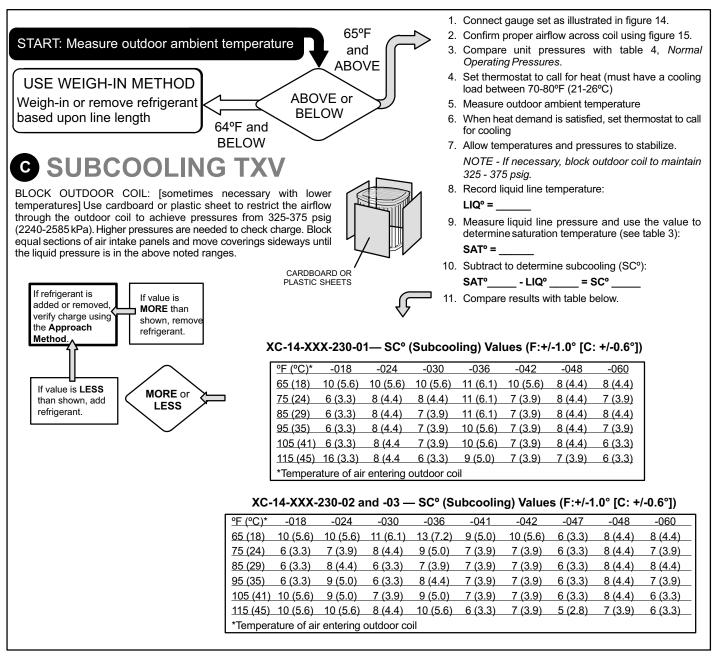
Figure 19. Using HFC-410A Subcooling (TXV) Charge Method
