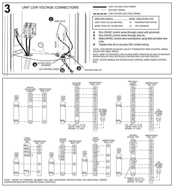
Figure 13. 24VAC Control Wiring Diagrams (Field Installed)
