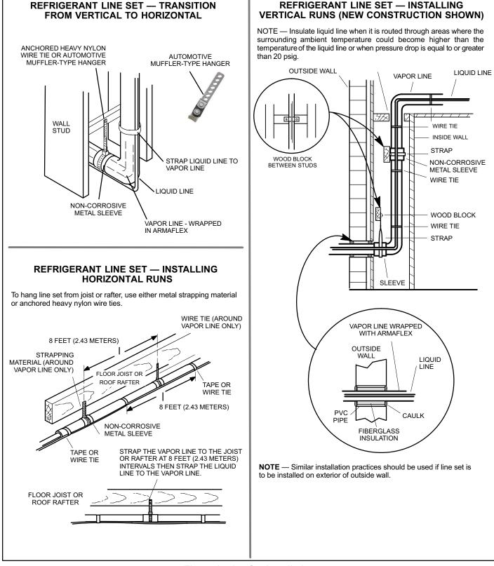
Figure 6. Line Set Installation
