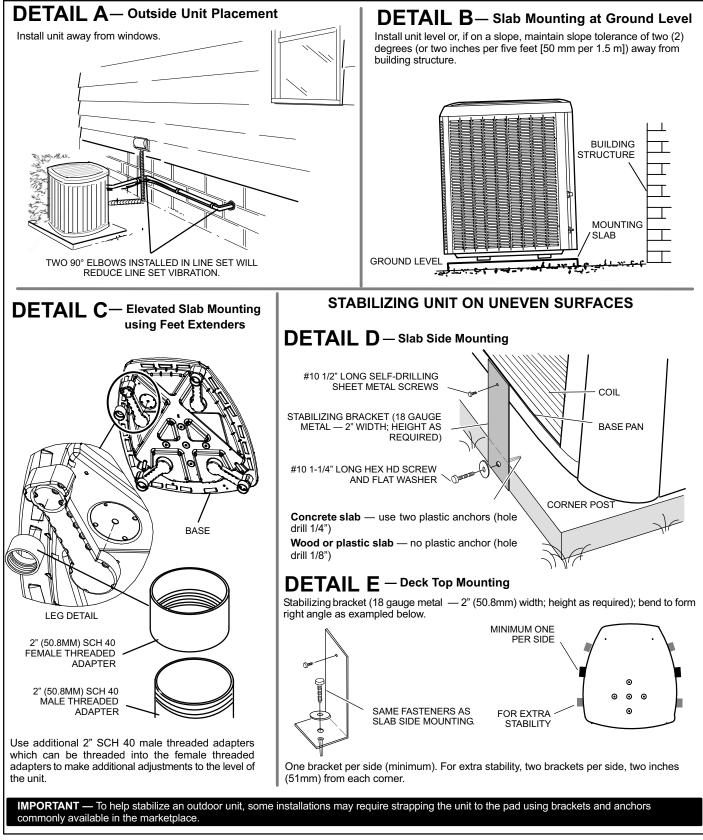
Figure 4. Placement, Slab Mounting and Stabilizing Unit
