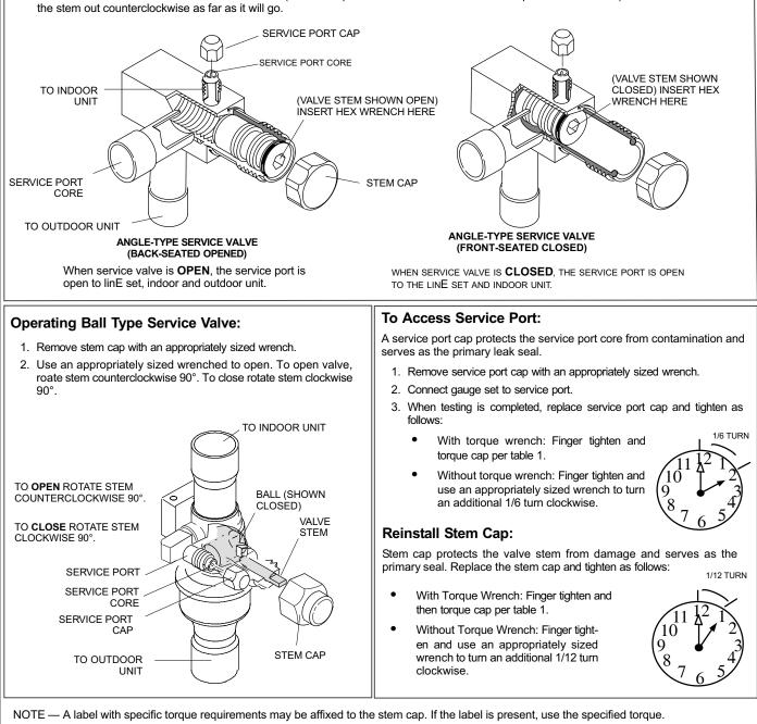
Figure 2. Angle and Ball Service Valves
