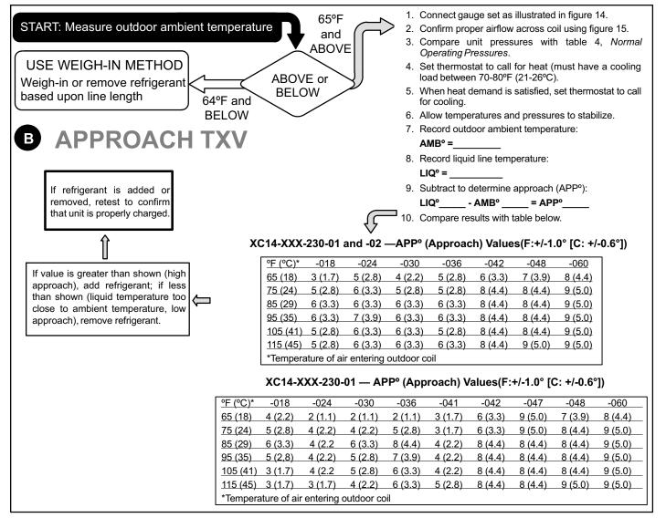
Figure 18. Using HFC-410A Approach (TXV) Charge Method
