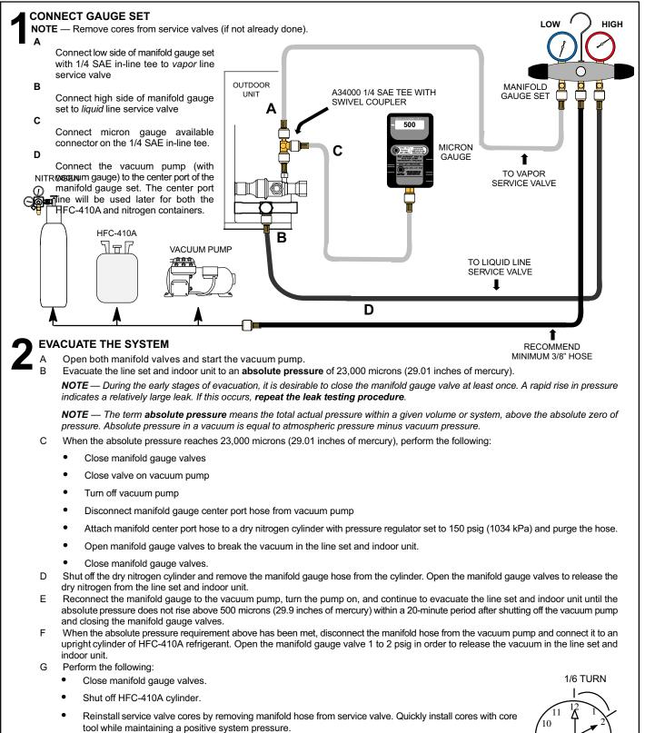
Replace stem caps and secure finger tight, then tighten an additional one-sixth (1/6) of a turn as illustrated.
