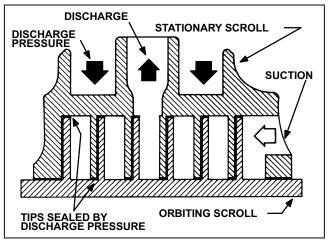
Figure 5. Scroll Cross-Section
