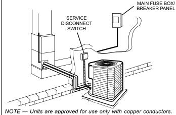
Ground unit at disconnect switch or to an earth ground.
