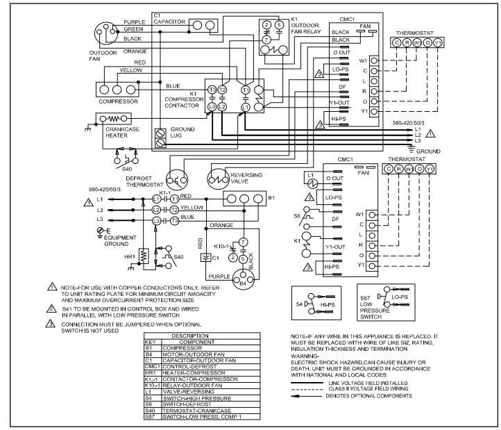
Figure 19. Typical Field Wiring Diagram — M Voltage — 380/420v (3PH) 50Hz
