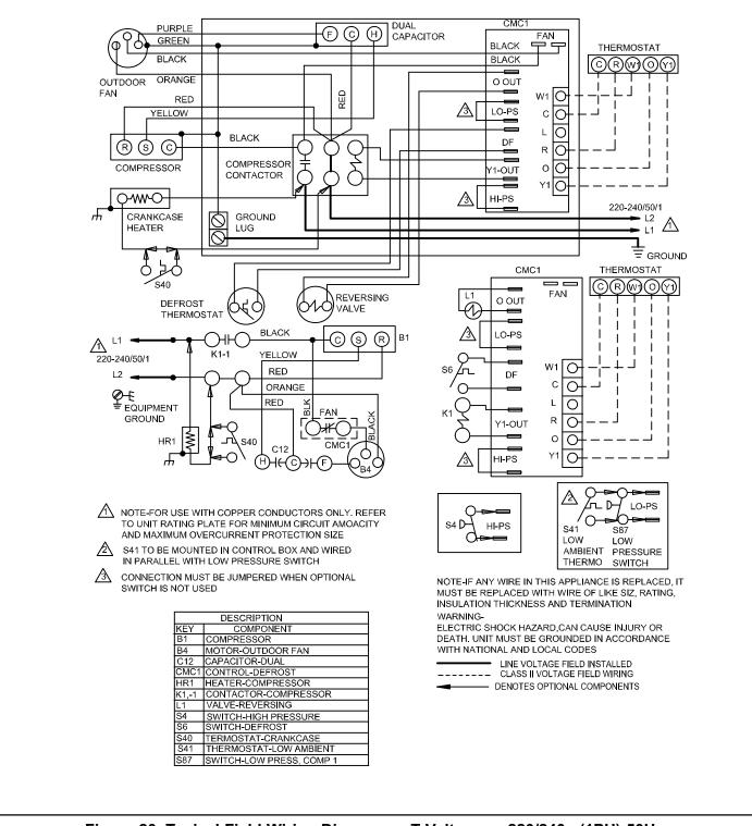
Figure 20. Typical Field Wiring Diagram — T Voltage — 220/240v (1PH) 50Hz
