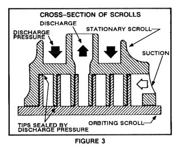
The counterclockwise orbiting scroll draws gas into the outer crescent shaped gas pocket created by the two scrolls (figure 4 - 1). The centrifugal action of the orbiting scroll seals off the flanks of the scrolls
