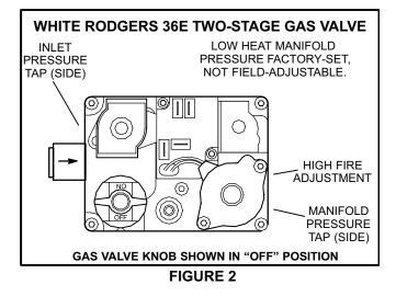
6 - Perform the following to **both** gas valves: turn knob on gas valve 180° either way to **OFF.** Do not force.
