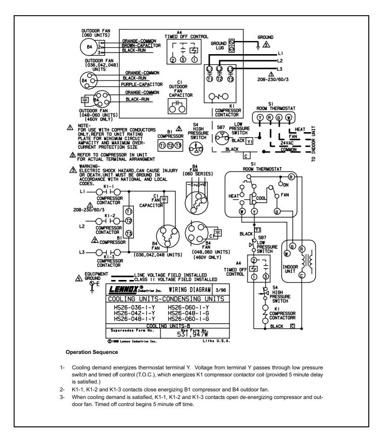
NOTE-Three-phase compressors must be phased correctly. Compressor noise will be significantly higher if phasing is incorrect. Compressor will operate backwards so unit will not provide cooling. Continued backward operation will cause compressor to cycle on internal protector.
